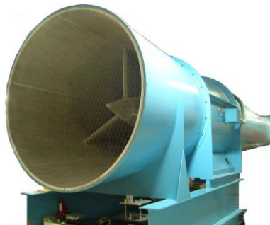
Noise-attenuating Exit Cone with Motor Nacelle
